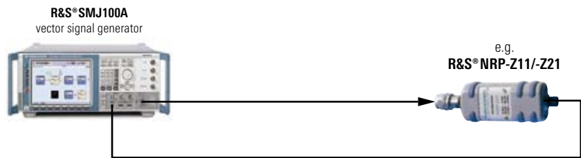
Automatic level correction for the R&S®SMJ100A signal generator using the R&S®NRP-Z11/-Z21 terminating power sensor
